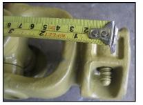
Required length of shaft is groove to groove length (step 1)
