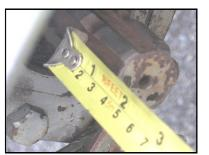
Remove safety guard from new shaft and measure length between shaft lock buttons or clamp bolts with shaft in closed position.
