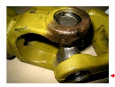
**IMPORTANT:** Grease follows the easiest path through internal ports to the four cross bearings.
