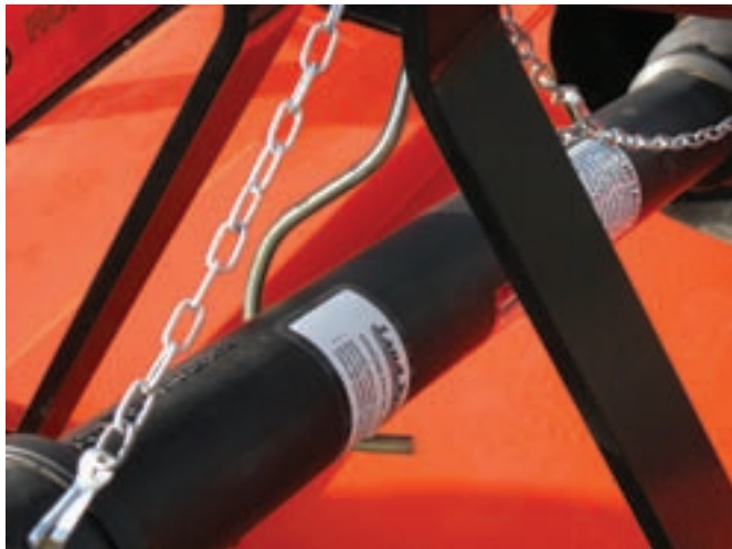
Figure 4: Hook-style PTO support.
